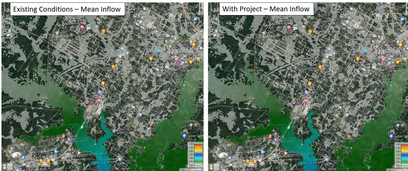
Figure E:14-16. 10-year 2082 event, Existing Condition (left) and With Project (right), depicting the change in WSE between the HSLR-LSLR simulations with mean inflows on the Pearl River and Bogue Chitto River; zoomed into Mile Branch project area
