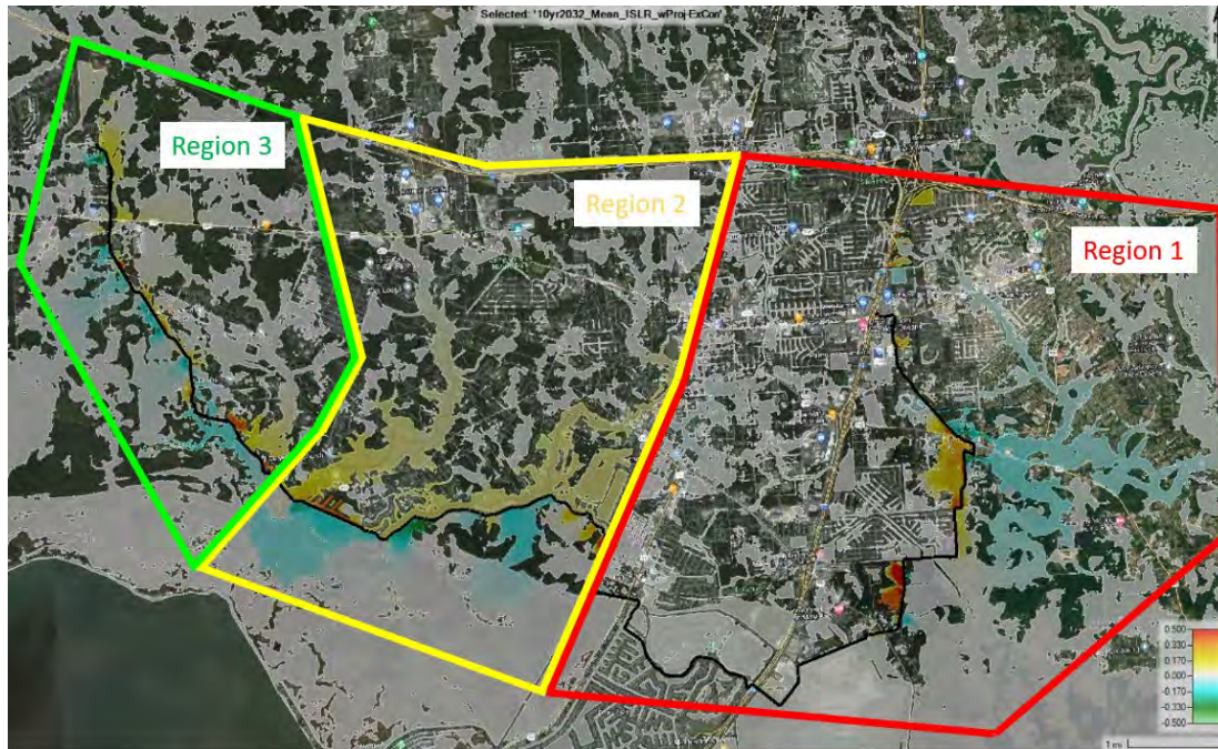
Figure E:14-6. 10-year 2032 event difference map depicting WSE increases and lowering's for the intermediate rate of SLR and mean inflows on the Bogue Chitto River and Pearl River. Regions correlate to areas discussed in the following results section. For a comprehensive description of difference maps refer to Annex 3 of this appendix.
