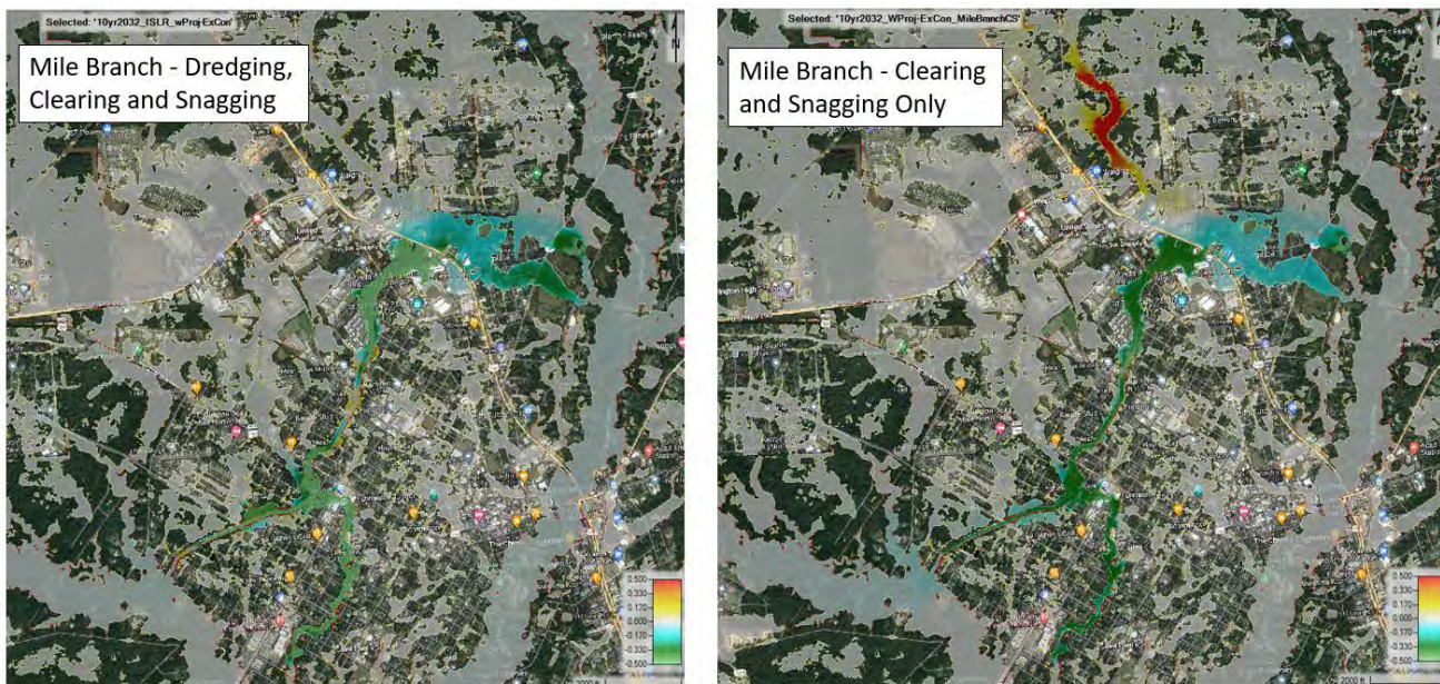
Figure E:14-3. Difference maps for the 10-year 2032 event with the intermediate sea level rise (ISLR) rate at Lake Pontchartrain, in the vicinity of Mile Branch comparing the Optimized_____ TSP with dredging, clearing and snagging of the channel (left) and only clearing and snagging of the channel (right).
